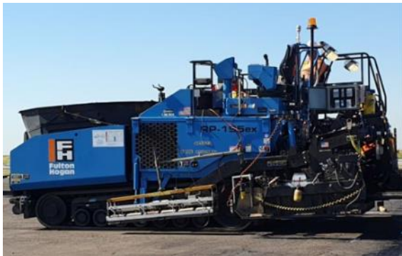
Figure A.3: Asphalt Paver (Roadtec RP-195ex)
